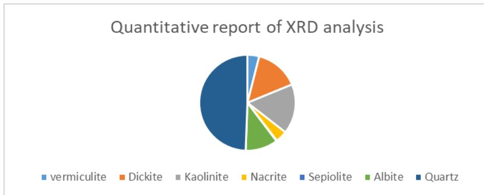
Fig. 4: XRD analysis of Calcined clay (Quantitative)
