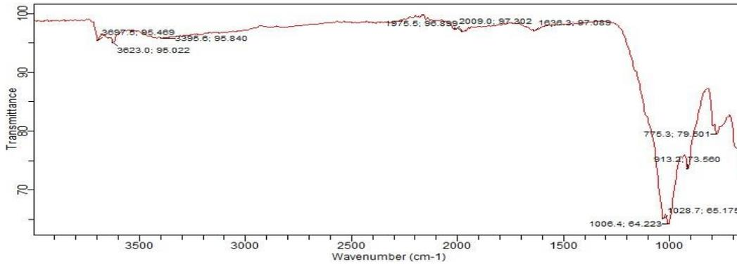
Fig. 6: FTIR Spectroscopic analysis of Calcined Clay
