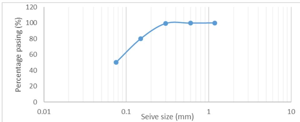
Fig. 3: Grading curve of Calcined Clay
