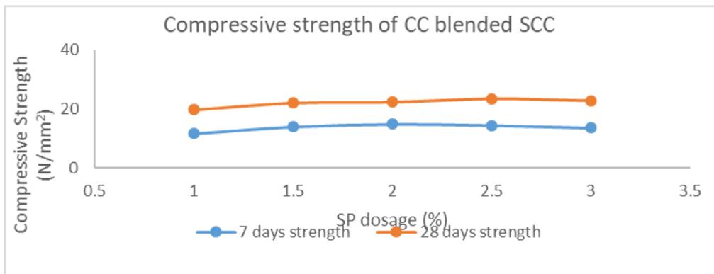
Fig 8: relationship between Compressive Strength and SP dosage
