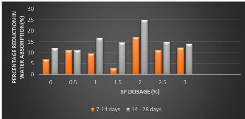
Fig. 9: Change in water absorption with age
