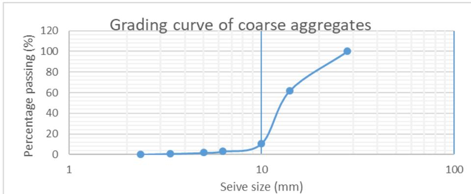
Fig. 2: Grading curve of coarse aggregates
