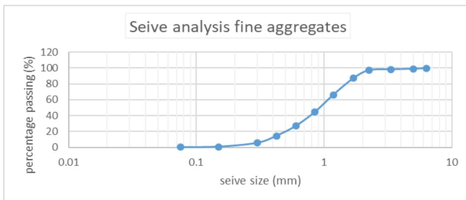
Fig. 1: Gradation curve for fine aggregates
