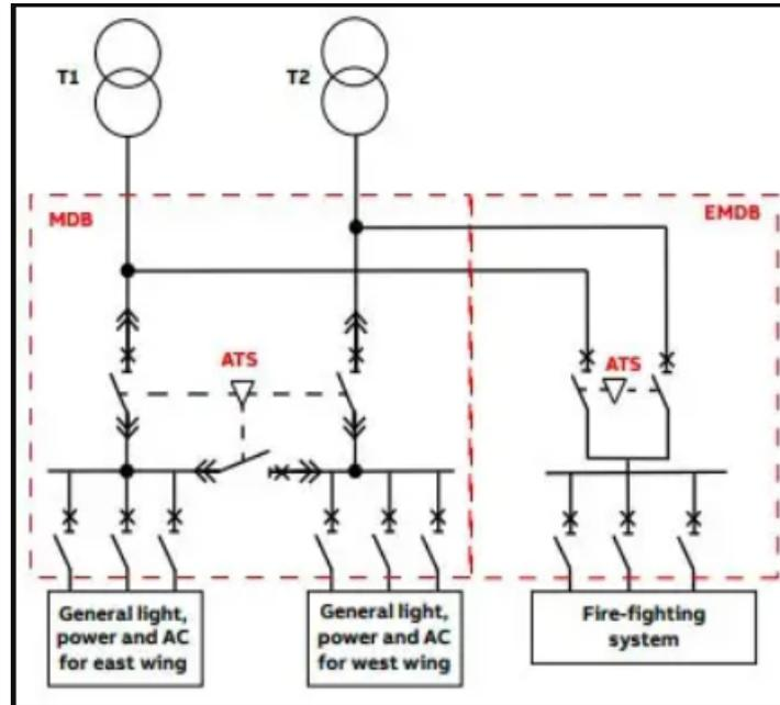
Fig. 2. ATS backing up supply for loads [4]
