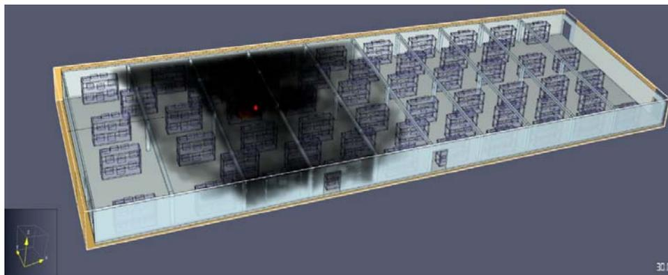
Fig. 7. Smoke propagation in the warehouse after 30 seconds
