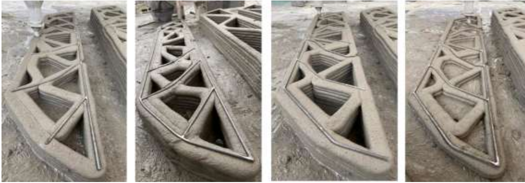
Fig 10 Reinforcement placement for different configurations. [10]
