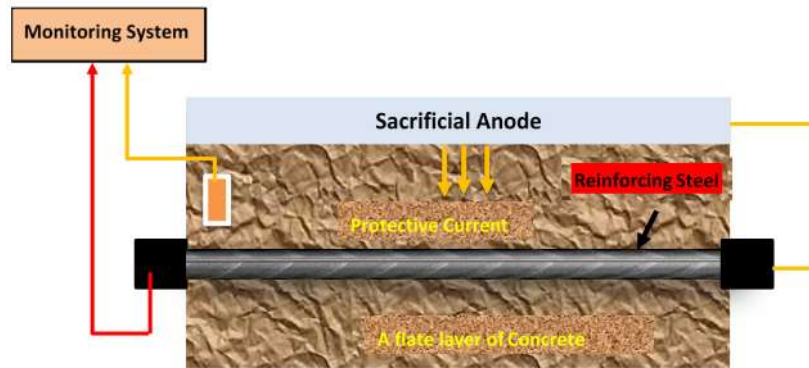
Fig 19 Sacrificial anodic cathodic protection structure schematic [15]
