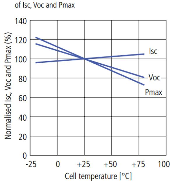
Fig. 1. The influence of temperature over conversion efficiency [1]
