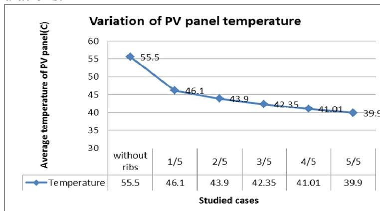
Fig. 4. Average temperature of PV panel for different  $h/S$  values
