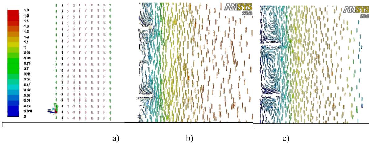
Fig. 7. Velocity magnitude for cases: a) without ribs; b)  $h=1$  cm; c)  $h = 2$  cm
