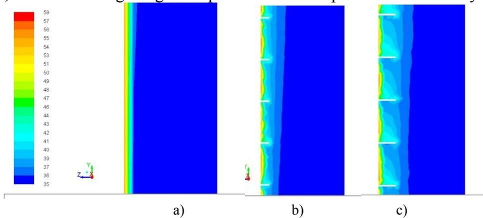
Fig. 5. Temperature spectra for cases: a) without ribs; b)  $h=1$  cm; c)  $h = 2$  cm
