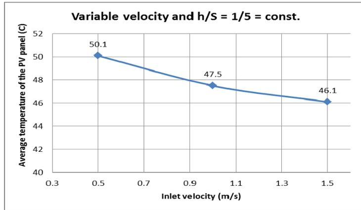
Fig. 3. Variation of PV panel temperature (interior surface) for different inlet velocities
