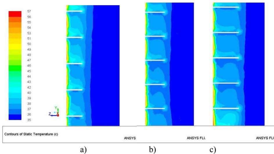
Fig. 6. Temperature spectra for cases: a)  $h = 3$  cm; b)  $h = 4$  cm; c)  $h = 5$  cm
