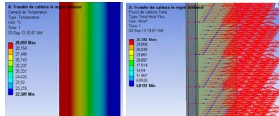
Fig. 12. Heat transfer simulation results for temperatures (left) and total heat flux (right), summer season in case of double pane window
