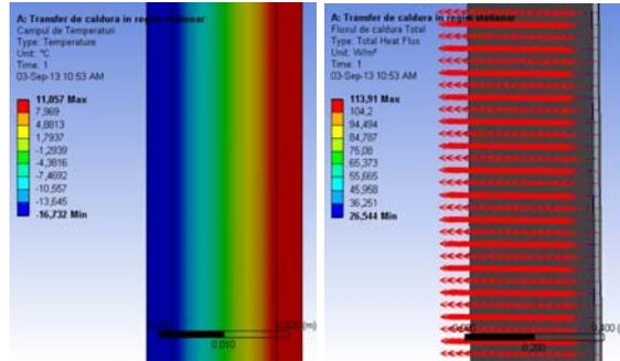
Fig. 11. Heat transfer simulation results for temperatures (left) and total heat flux (right), winter season in case of double pane window
