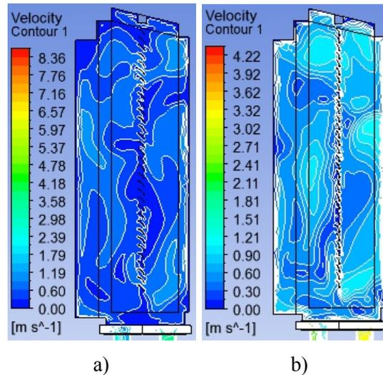
Fig. 4. Velocity contours inside cavity in case of shading slats positioned at 45° (a) and at 65° (b)
