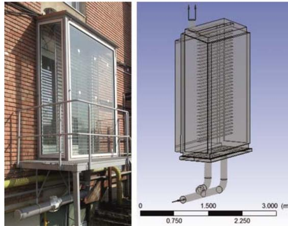
Fig. 1. Box double-skin façade experimental model (left). Simulation model in 3D (right)
