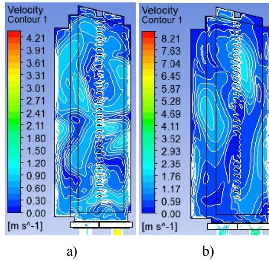
Fig. 3. Velocity contours inside cavity in case of shading slats positioned at 0° (a) and at 25° (b)
