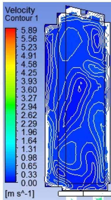
Fig. 2. Velocity contours inside cavity in case of shading system fully rose
