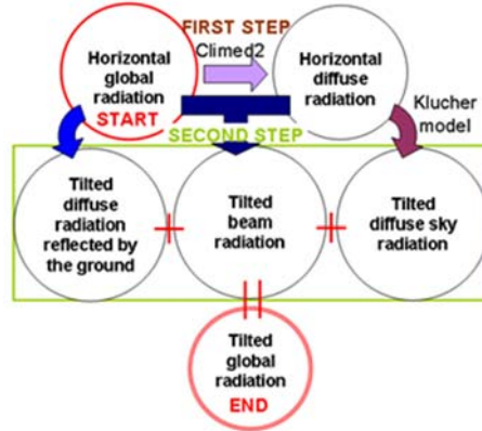
Fig. 7. Method for determining the solar radiation on an arbitrary oriented and tilted surface from horizontal one.
