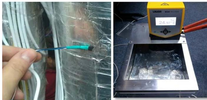
Fig 4. a) TSic T501 sensors used for the measurement and control part of the thermal manikin , b) thermostatic water bath Lauda Eco with immersion thermostat Lauda Eco Silver
