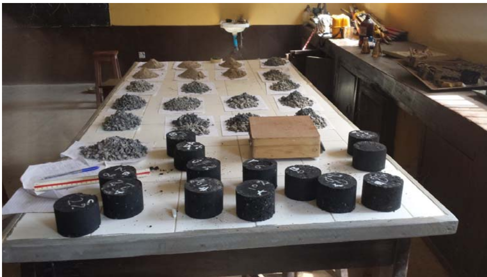
Plate 3. Air curing of the asphalt samples
