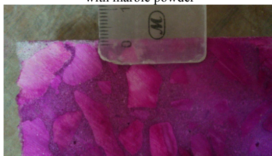
Fig.6. Determination of Carbonation depth with phenolphthalein pulverisation
