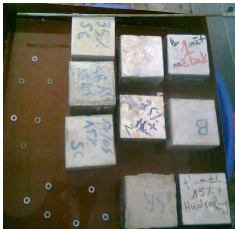
Fig.6. Water absorption test on concrete cubes
