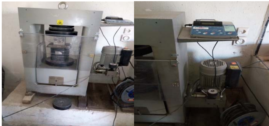
Fig.2. Machine for compressive strength test.
