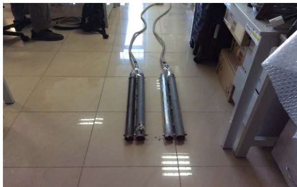
Fig. 5 Non-galvanized and galvanized metal samples with senzors
