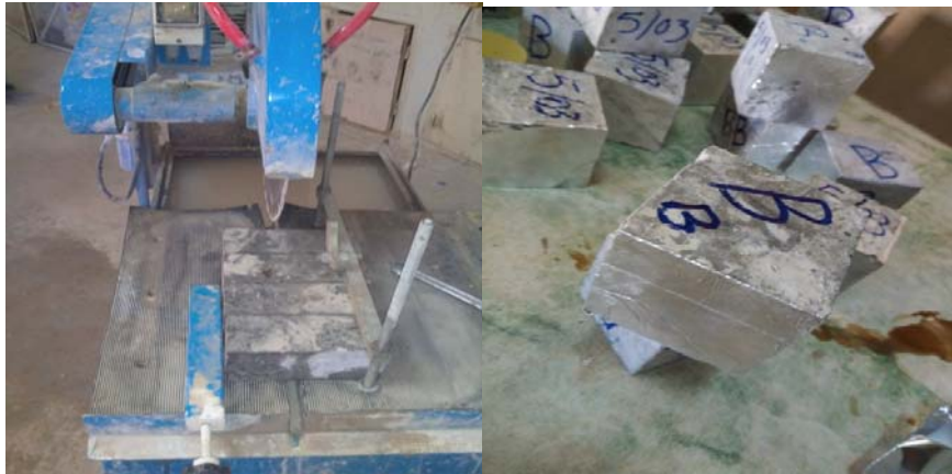
Fig. 4.: Preparation of Samples for accelerated carbonation test.
