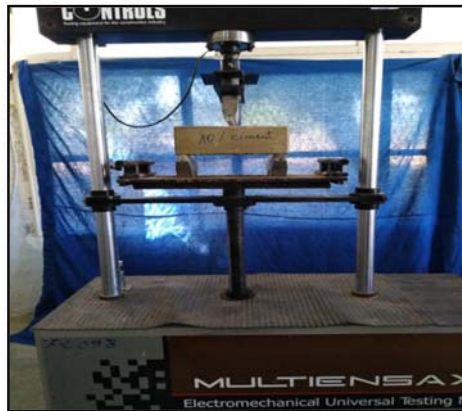
Figure 6: flexural strength test.
