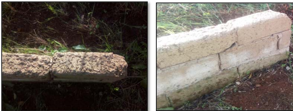
Figure 14: Wall condition stabilized by 10% lime (November 2020).
