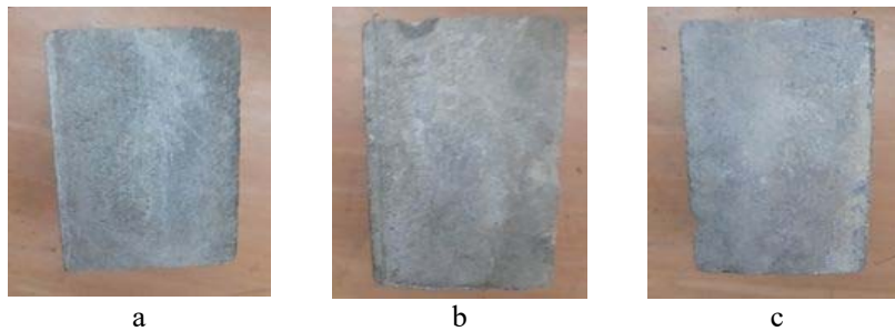
Fig. 1. Appearance images of gypsum-based composite a – version 1; b – version 2; c – version 3.
