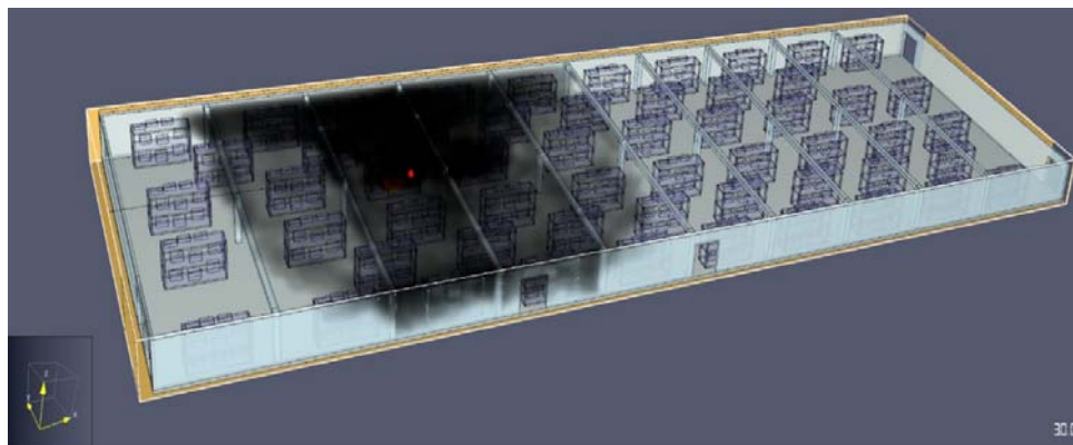
Fig. 7. Smoke propagation in the warehouse after 30 seconds
