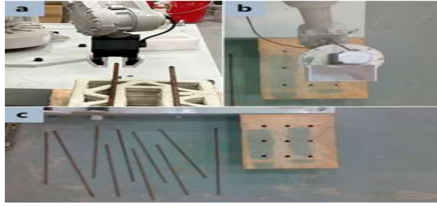
Fig 5 Experimental setup. (a) Gripper; (b) Concrete extruder; (c) Rebars and printing base. [5]
