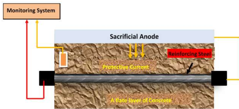
Fig 19 Sacrificial anodic cathodic protection structure schematic [15]
